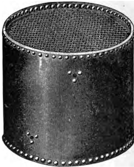
FIG. 337.—Another type of Small Carriage Boiler, showing both tube plates inlanged and riveted to a seamless steel tube.
